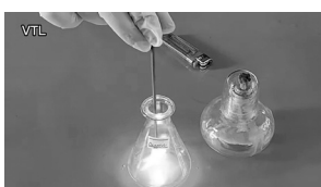
Figure 3. Red embers ignite after being put into the Oxygen tank
