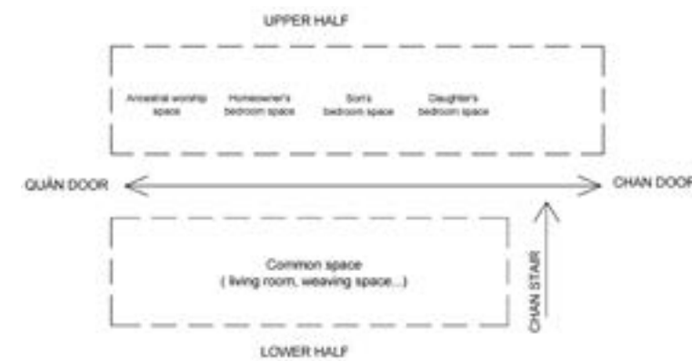
Figure 23. "The common layout method for space utilization on the second floor of the Thai Den stilt house in Tram Tau"
