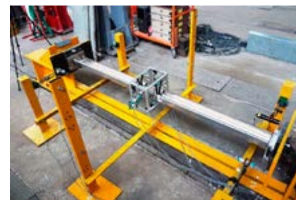
(a) The compression test rig
