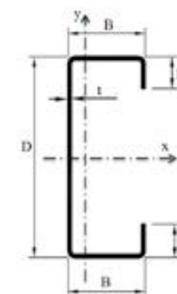
Figure 2. The nominal dimensions of the channel section
