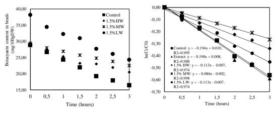
*Figure 7.* Diagram of the degradation kinetics of betacyanins in extract and encapsulated beads; (■)alginate; (▲)betacyanins extract; (♦)1.5% LW chitosan-alginate; (★)1.5% MW chitosan-alginate; (●)1.5% HW chitosan-alginate.
