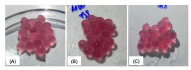
*Figure 8.* Betacyanins encapsulated in chitosan-alginate beads. (A) LW chitosan-alginate; (B) MW chitosan-alginate; (C) HW chitosan-alginate.
