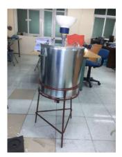
Figure 7: Completed set of rainwater collector for stable isotope analysis
