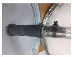
Figure 5a: The connection between container cap and drainage pipe
