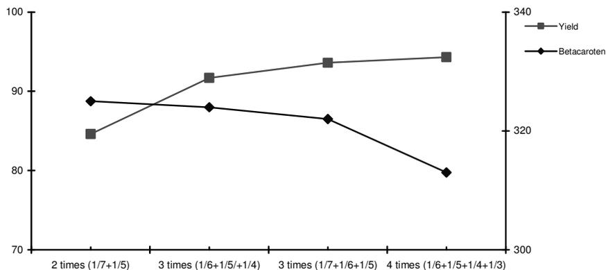
Figure 2. Effect of numbers of extractions and solvent amount on the extraction yield and beta-caroten content
