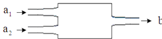
Figure 8. Structure of an OR logic gate based on a 2 \times 1 SI-MMI coupler
