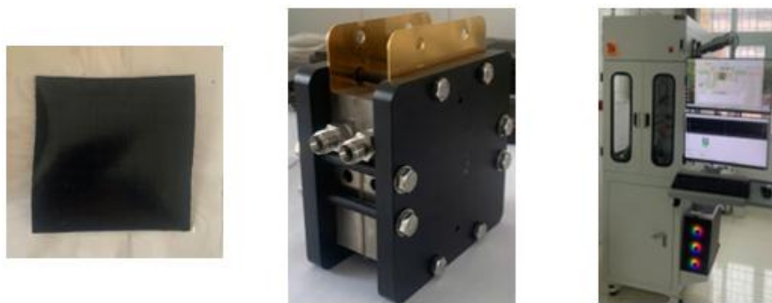
Fig. 2. MEA membrane electrode (a); PEMWE single electrolyzer (b); 500 W electrolyzer evaluation system-Scitech Korea (c).
