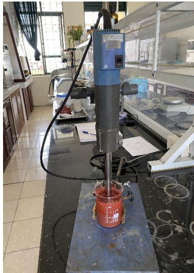
Fig. 1. Nano additive is dispersed into the binder solution.
