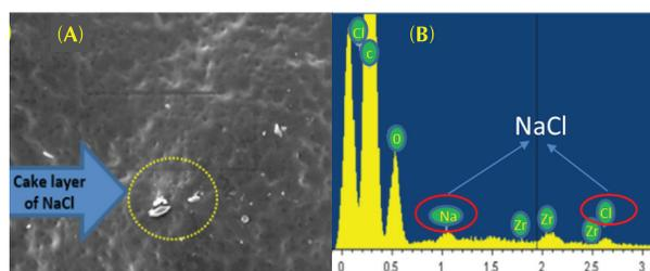
Fig. 6. (A) SEM picture and (B) EDS graph of a used membrane (0.3 M EDTA-2Na coupled with 0.6 M NaCl as draw solute, 6000 mg NaCl/l as feed solution, draw solution facing the support layer, pH of 8, temperature of 25±0.5°C).
