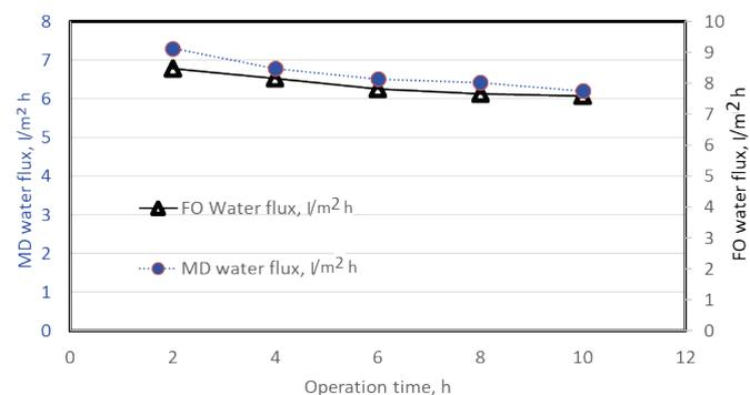
**Fig. 5. Variation of FO water flux and MD water flux for the desalination of brackish water versus operation time (0.3 M EDTA-2Na coupled with 0.6 M NaCl as draw solute, MD membrane: PTFE 0.45 µm; hot stream: 55±0.5°C; distillate stream: 25±0.5°C).**
