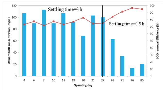
Fig. 4. COD removal performance in the PBR with different settling time.
