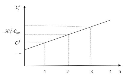
Fig 2. The  $C_t^2$  versus the change of the intensity of the neutron source
