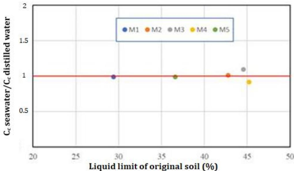
Figure 6. Relationship between the ratio of  $C_c \text{ seawater} / C_c \text{ distilled water}$  and the liquid limit of the original soil.
