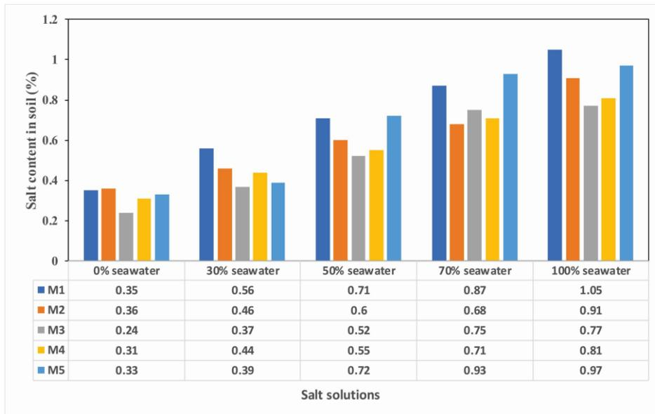
Figure 1. Variation of salt content (%) in the soil after submerging in different salt solutions.
