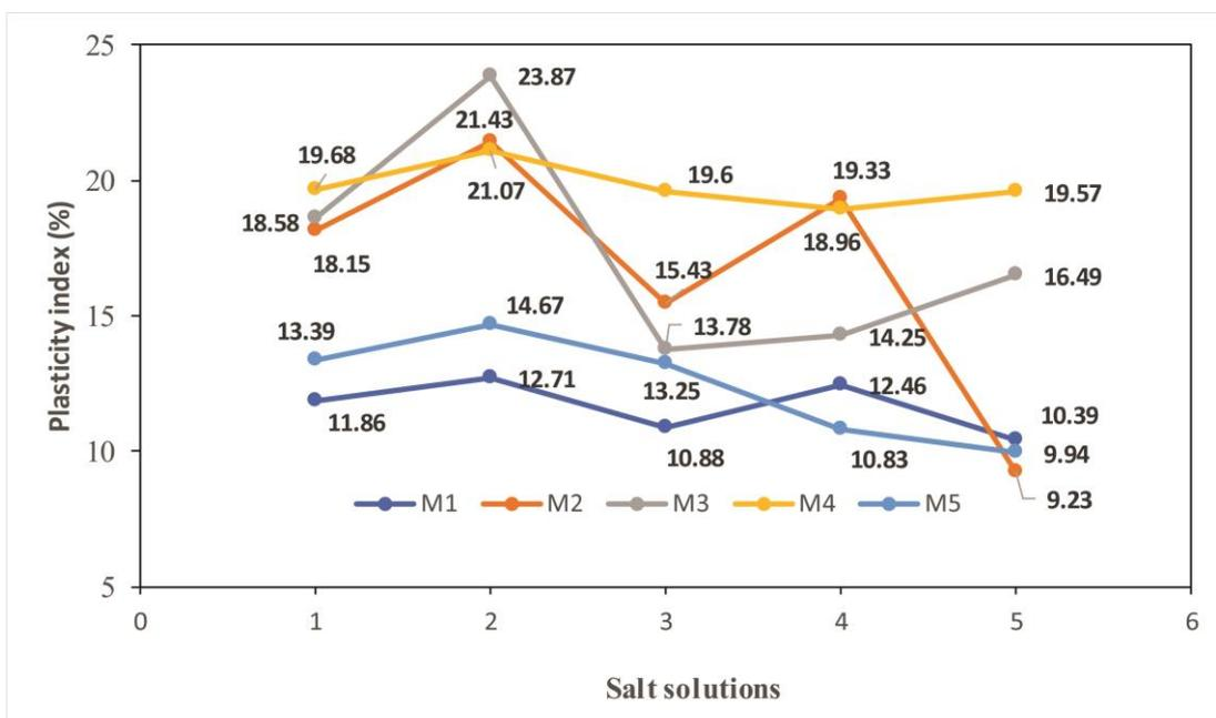
Figure 3. Variation of the plastic limit of soil in different seawater solutions.
