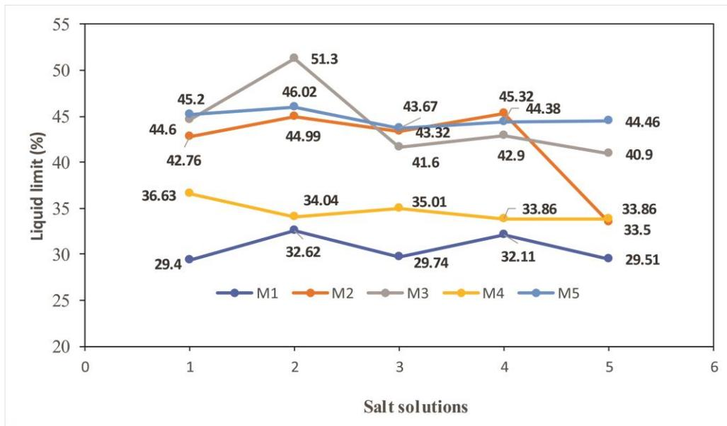
Figure 2. The variation of the liquid limit in different salt solutions.
