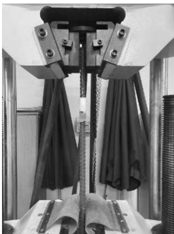
Figure 3. Tensile test of corroded reinforcing bar
