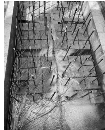
Figure 2. Test Samples when corrosive with salt electrolyses NaCl 3,5%
