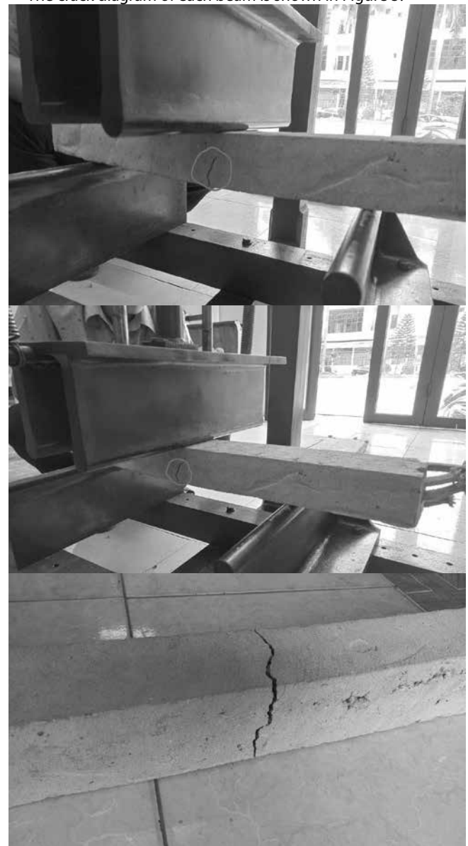
Figure 5. Crack pattern for the tested beams
