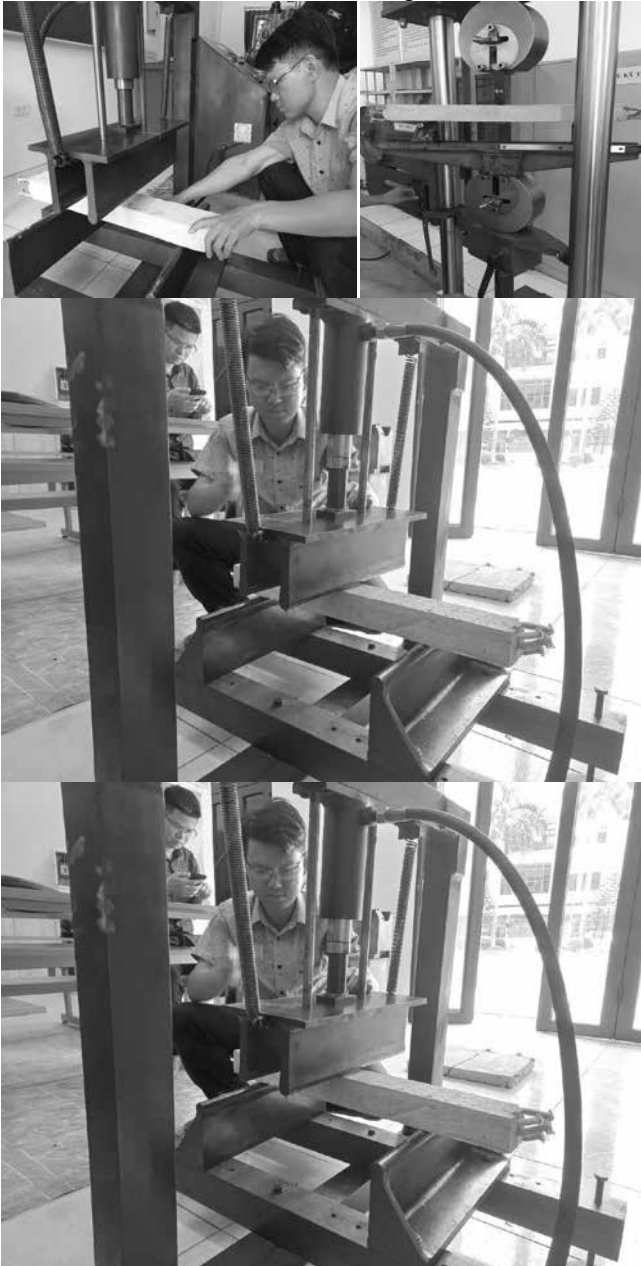
Figure 3. Bending test of concrete beams reinforced with composite aramid bars Table 3. Summary of bending resistance of beams
