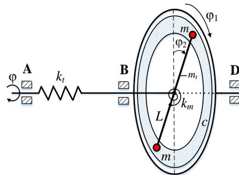
**Figure 1.** Shaft Model with Installed TMD
