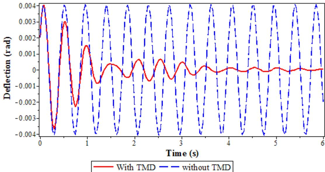
**Figure 4.** The vibration of the machine shaft with  $\theta_0 = 2 \times 10^{-3}(\text{rad})$  and  $\dot{\theta}_0 = 5 \times 10^{-2}(\text{rad} / \text{s})$  in the case of random excitation  $M(t)$
