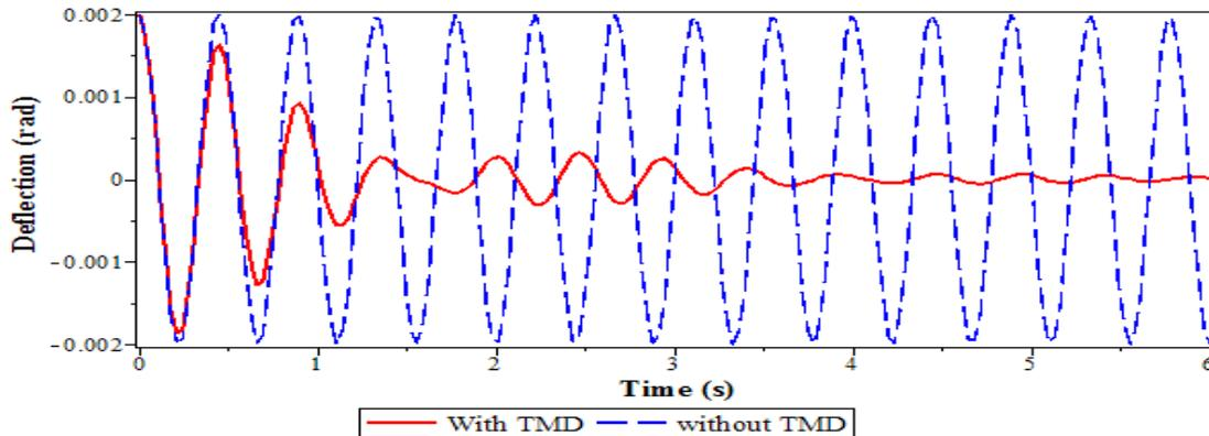
**Figure 2.** Vibration of the machine shaft with  $\theta_0 = 2 \times 10^{-3}(\text{rad})$  in the case of random excitation  $M(t)$
