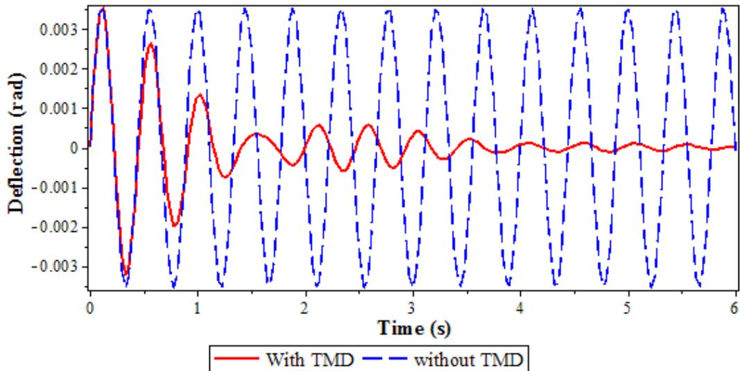
**Figure 3.** The vibration of the TMD with  $\theta_0 = 2 \times 10^{-3}(\text{rad})$  and  $\dot{\theta}_0 = 5 \times 10^{-2}(\text{rad} / \text{s})$  in the case of random excitation  $M(t)$
