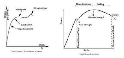
Figure 3. Tensile strength and yield elongation graph curve
