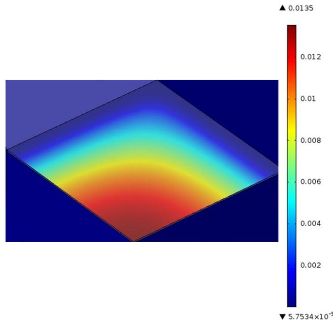
**Fig. 3:** Structure surface deflection of 3 layer graphene membrane when applied pressure of 10 Pa
