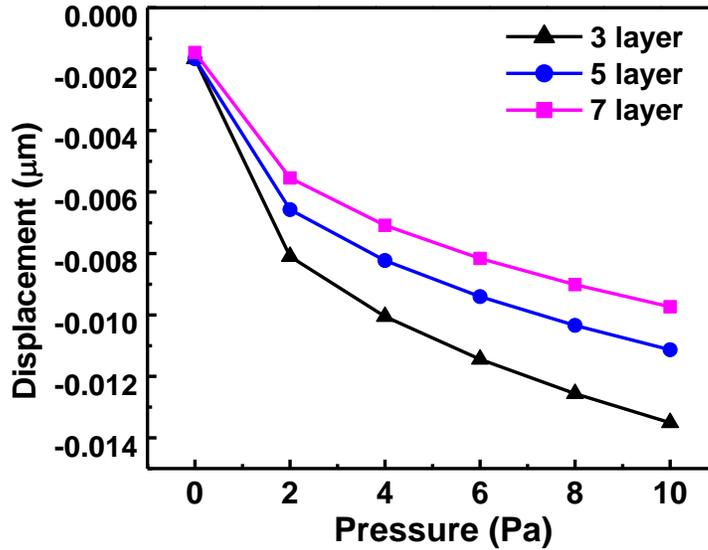
Fig. 4: Displacement of sensor with different thicknesses of membrane
