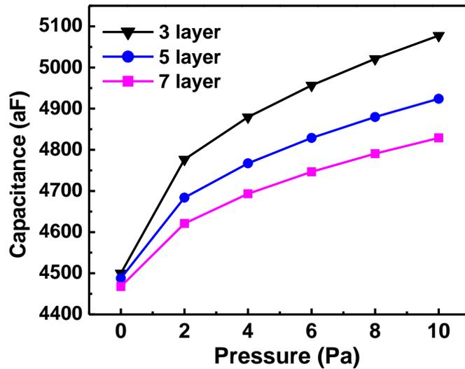
Fig. 5: Capacitance of the sensor when apply pressure
