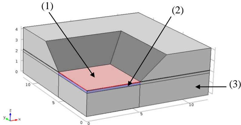
**Fig. 1:** The symmetric device geometry with one quadrant of pressure sensor, where: (1) graphene membrane, (2) air chamber, (3) silicon substrate.
