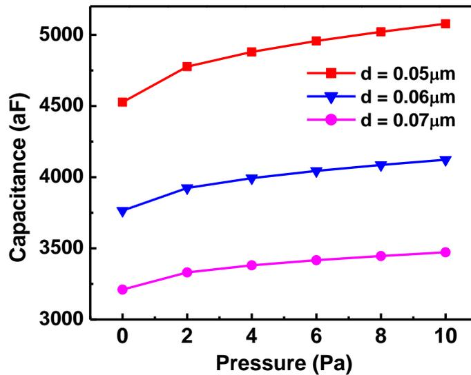
**Fig. 6:** Capacitance of pressure sensor with different thickness of air chamber
