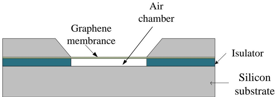
**Fig. 2:** The cross-sectional view of the MEMS capacitive pressure sensor
