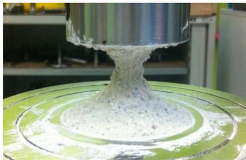
**Figure 1:** *A squeezing experiment of mortar in process*
