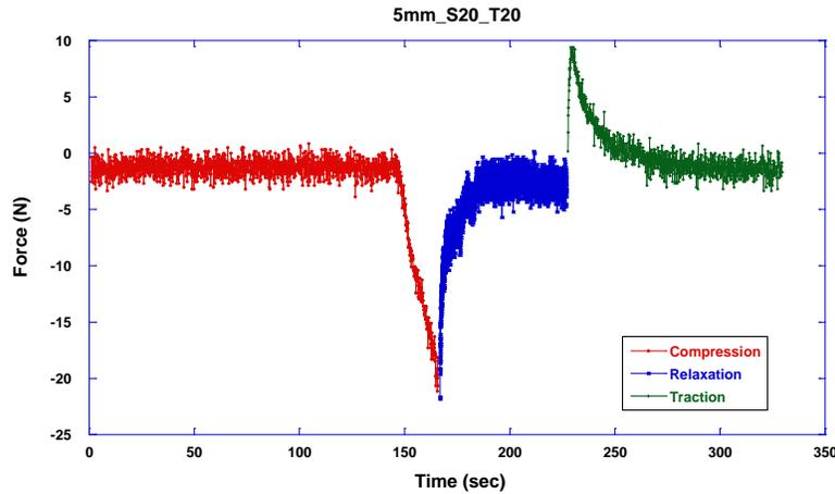
Figure 2: A typical curve obtained from a squeeze tack test
