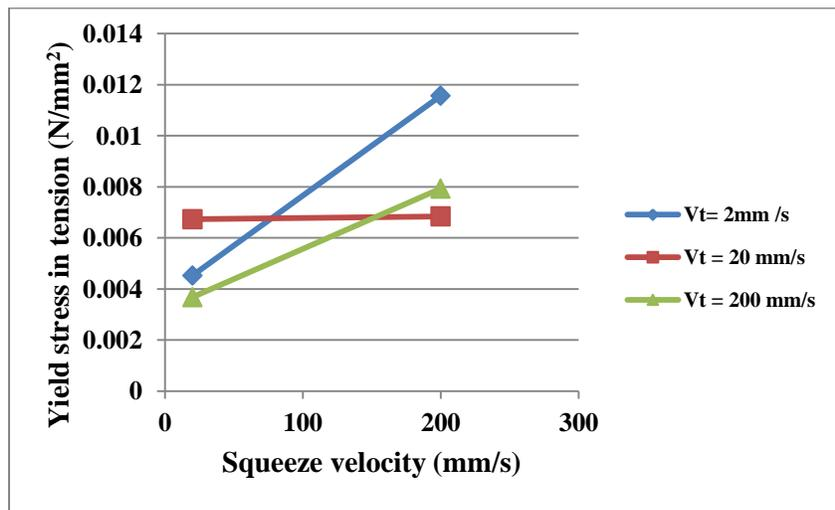
**Figure 5:** Calculated materials' yield stress versus squeeze rates at different tack velocities
