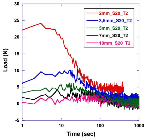
**Figure 4:** A typical curve obtained in the tack period of squeeze flow test
