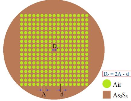
**Figure 1:** The geometrical structures of PCFs with square lattice and As<sub>2</sub>S<sub>3</sub> substrate
