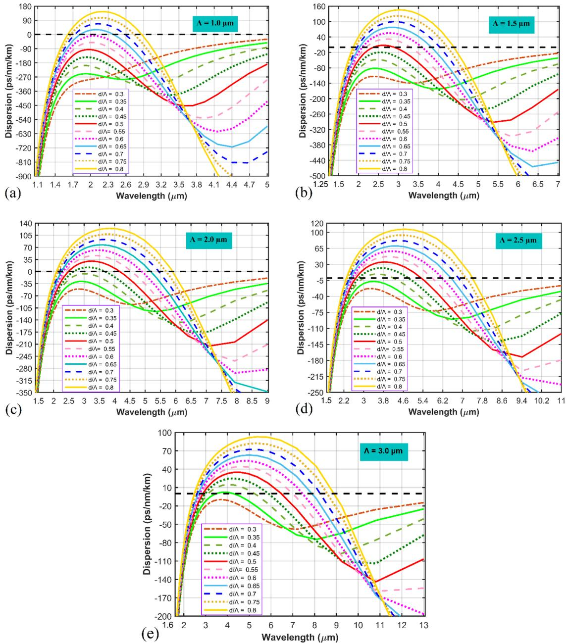
**Figure 2:** The chromatic dispersion of PCFs with various  $d/\Lambda$  for (a)  $\Lambda = 1.0 \mu\text{m}$ , (b)  $\Lambda = 1.5 \mu\text{m}$ , (c)  $\Lambda = 2.0 \mu\text{m}$ , (d)  $\Lambda = 2.5 \mu\text{m}$ , and (e)  $\Lambda = 3.0 \mu\text{m}$ .
