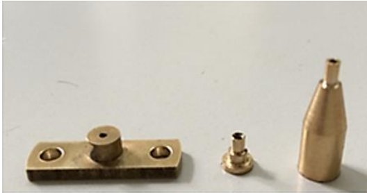
Figure 1: Components for coupling the radiation from diode laser to optical fibers. From left to right: heatsink submount; fixing disk; outer cap
