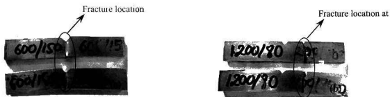
Figure 12. Fracture locations of weld regimes \omega/v = 4.0 rev/mm (a) and \omega/v = 15.0 rev/mm (b).
