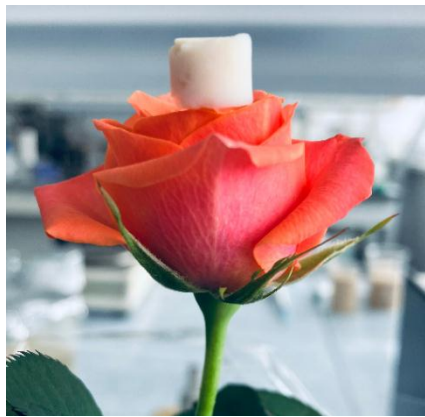
Fig. 3. Physical shape and light weight of a hybrid aerogel based on silicon dioxide and lignosulfonate.
