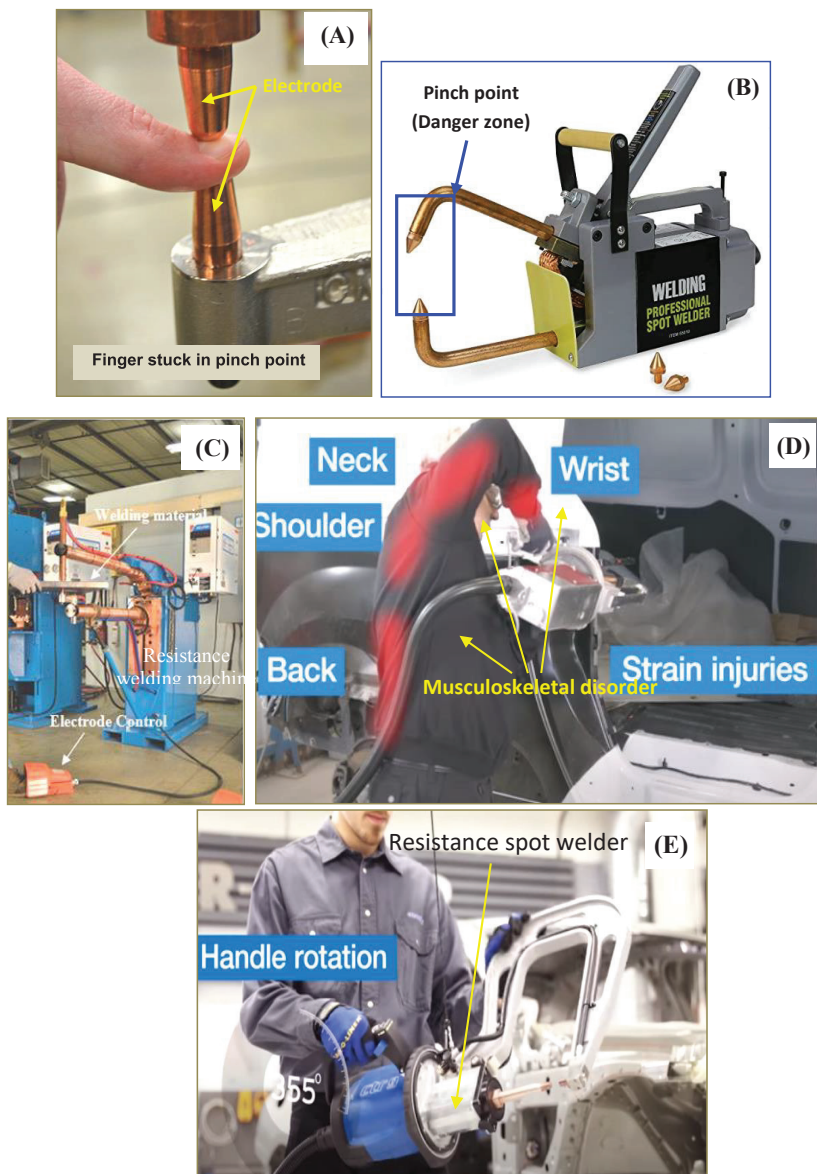
Fig. 4. (A) Finger caught between electrodes in resistance welding, (B) portable resistance spot welding machine with pinch point and danger zone, (C) welding of material with leg operation, (D) resistance welding hazards, and (E) advanced resistance spot welder (Car-O-Liner CTR9) with zero hazards.
