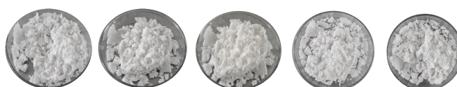
Fig. 6. Sample of calcium lactate during drying at 80°C for the first 5 hours.
