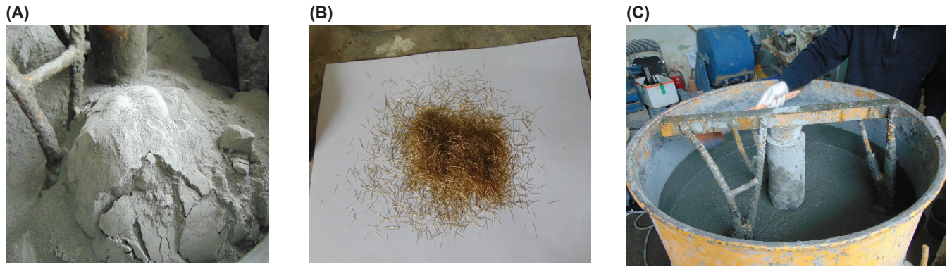
Fig. 17. Photos of (A) Cementitious matrix, (B) Steel fibres reinforcement, and (C) Mixing procedure of ultra-high performance concrete.
