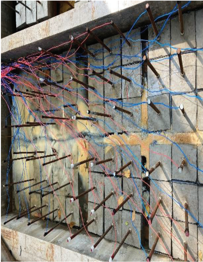
Fig. 2. Test samples when corrosive with salt electrolyses NaCl 3.5%.
