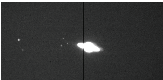
Fig. 5. Field of view (FOV) of the spectrograph through the guider. The black line in the middle represents the slit. The light from the object that the slit is pointing to will enter the spectrograph; in this case, it is light from the ring of Saturn.
