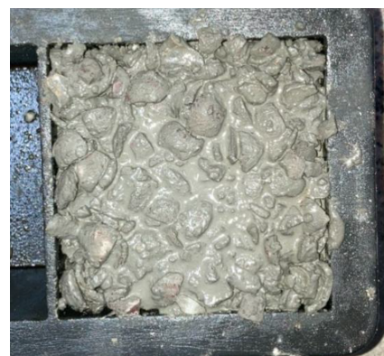
Figure 4. Concrete specimens 100mmx100mmx100 mm
