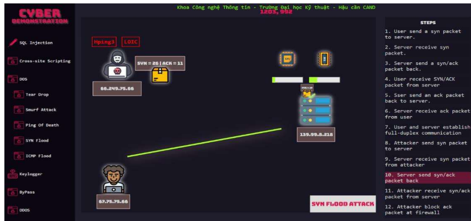
Figure 7. Illustration interface of the SYN Flood attack technique
