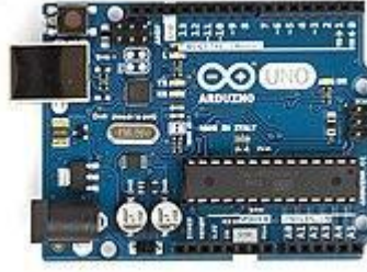
Figure 3. Arduino microcontroller and ADC conversion module.
