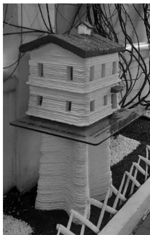
Figure 13. The villa was built with a 3D concrete printer.
