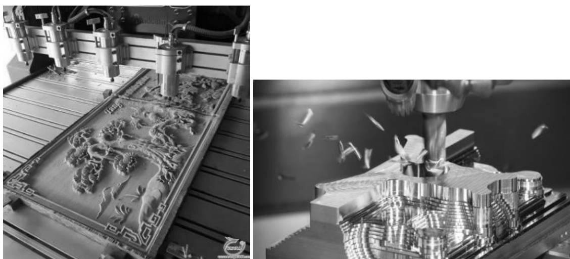
Figure 1. Steel and wood products after being engraved by a CNC machine [4, 5]
