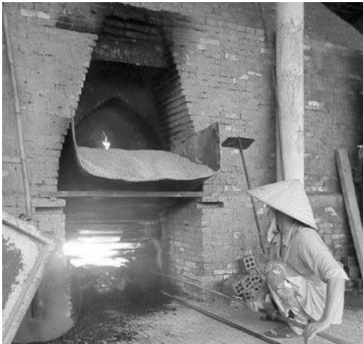
Figure 1. Burning rice husks in a ceramic kiln (Photo Credit: baovinhlong.com)
