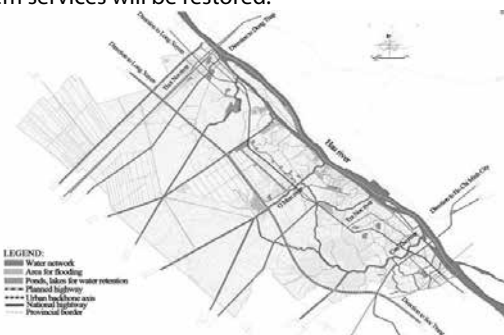
Figure 8. The new water infrastructure built on the existing water network enhances flood containment and drainage capacity with natural floodplains, regulating lakes, flooded parks and artificial water purification systems. The new water infrastructure helps the city strengthen flood resilience and restore river ecosystem services. Source: SIURP (2011)
