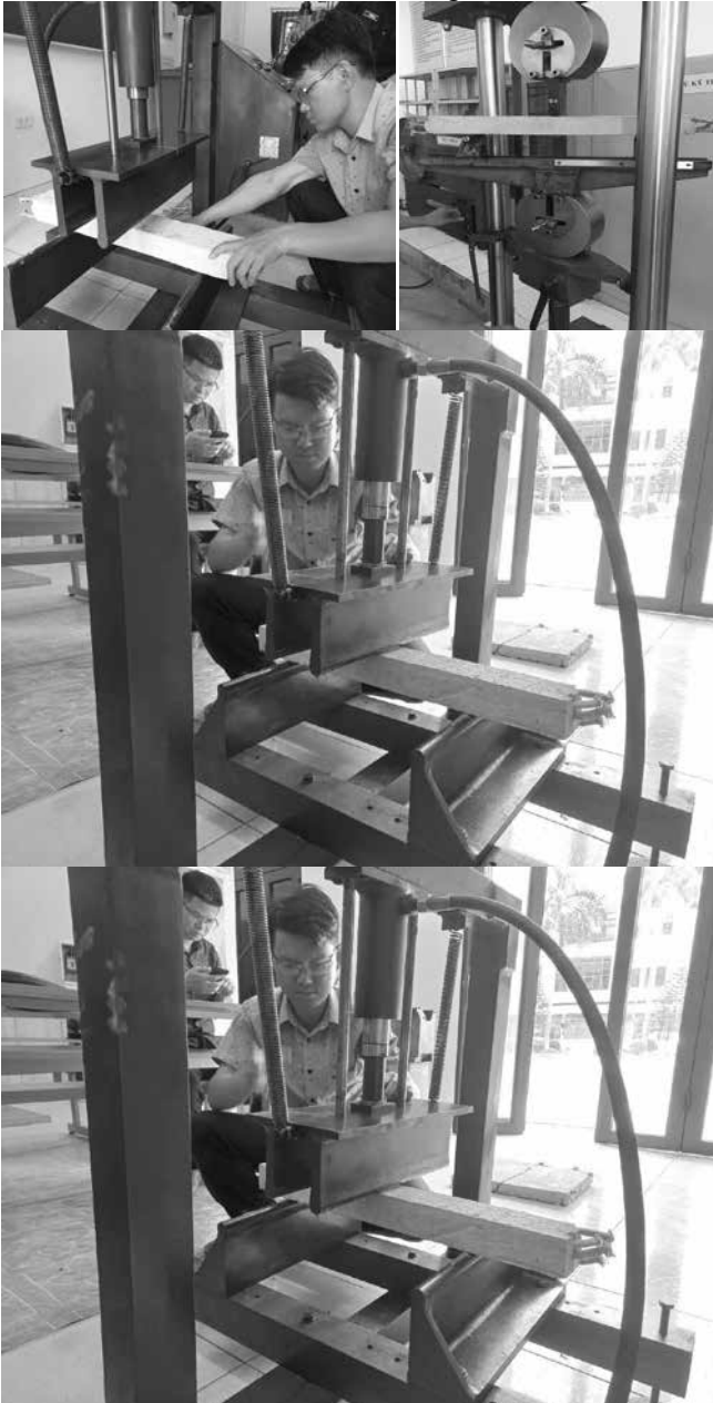
Figure 3. Bending test of concrete beams reinforced with composite aramid bars
