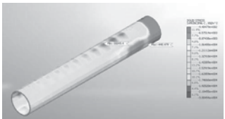
Figure 26: Minimum principal stress of the segment in S17
