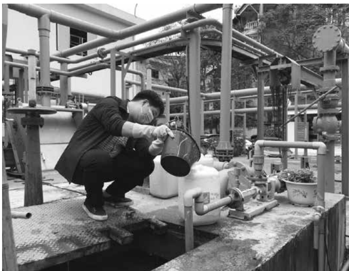
Figure 3. Wastewater collection at Truc Bach wastewater treatment - Hanoi
