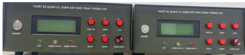
Figure 9. Image of two on-site monitoring and warning devices
