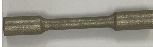
Figure 1. Image of the 3D printed Ti64 alloy tensile testing sample
