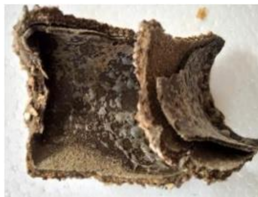
Figure 6. Ceramic shell showing swelling and delamination defects
