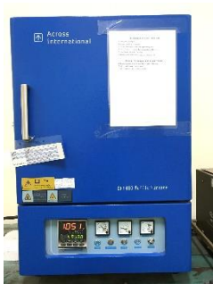
Heat Treatment Furnace
