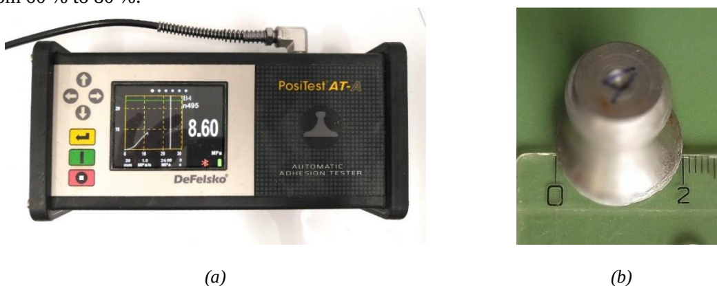
Figure 4. Pull-off device (a) and dolly (b)
