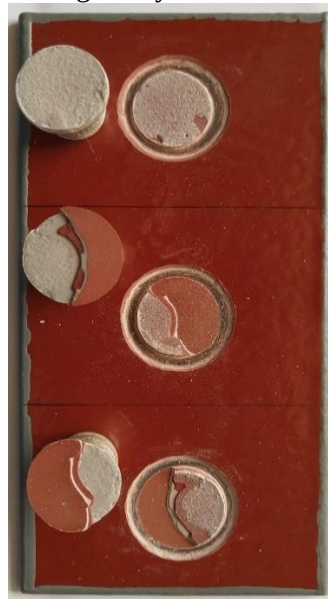
Figure 5b. Image of destruction on second coating (sample TMP3)
