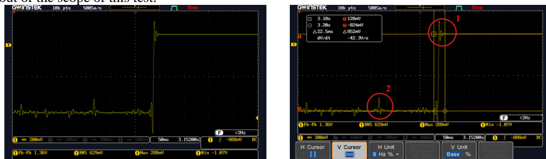
Figure 6. Real-time charge to discharge response
