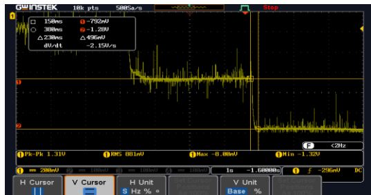
c) Charging response when charging power changes from 51.2 W to 76.8 W
