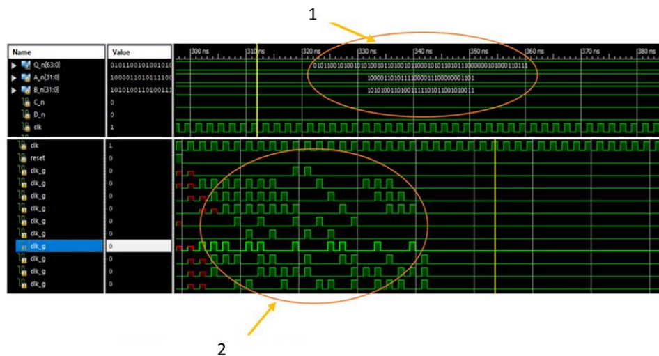
Figure 5. The waveform of the 32-bit pipelined multiplier when applying fine grain LACG technique in case of randomly generated A, B inputs
