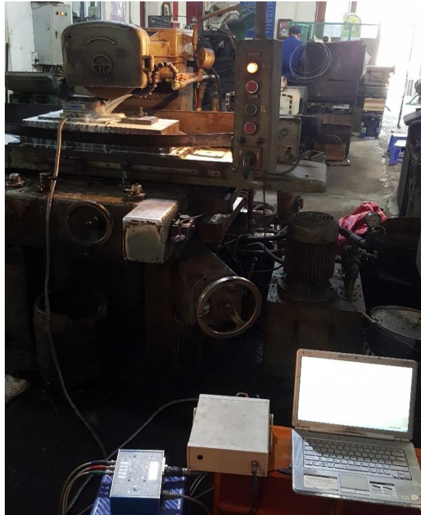
Figure 3. The actual connection measures the cutting force
