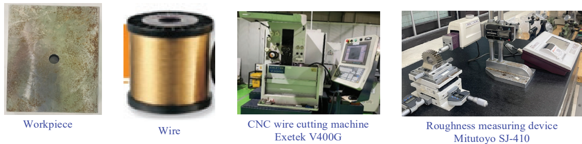
Figure 1. Workpiece, wire, machine in machining of non-circular gears, and tooth surface roughness meter
