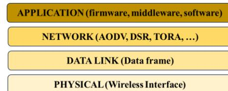
Figure 5. Layer structure of the mesh LoRa node
