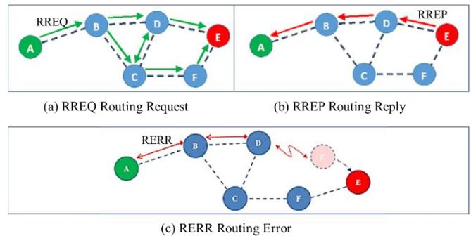
**Figure 4.** Example of AODV algorithm
