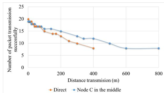
Figure 9. Number of packet transmission successfully vs. distance
