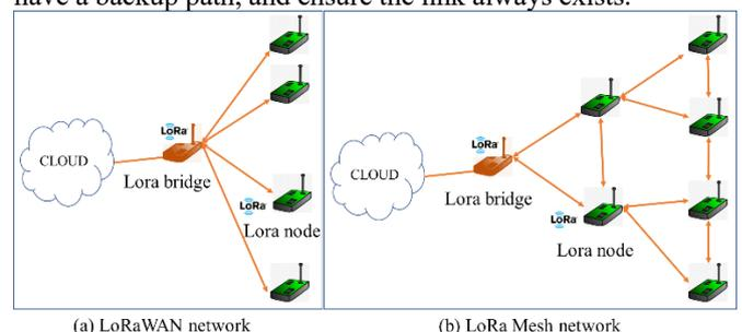
**Figure 1.** LoRa with a mesh network structure
