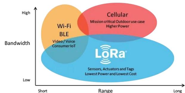
**Figure 2.** CSS in LoRa in comparing with other wireless technology of Bagur and Chung (2023)
