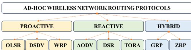
**Figure 3.** Classification of classical routing protocols
