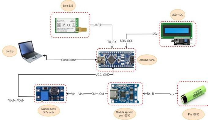
Figure 6. Block diagram of the mesh LoRa node
