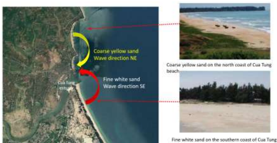
Figure 5: Diagram illustrating the mechanism of sediment transport in Cua Tung beach area
