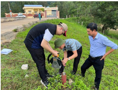
Figure 7: Measuring and checking the saturation line of Ham Lon dam at the site
