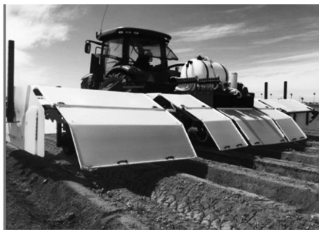
See and Spray technology, developed by John Deere and Blue River Technology, uses machine learning to identify weeds and spray chemicals only where needed.
